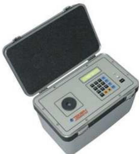
Figure C.2. The Tekran 2505 Mercury Vapor Primary Calibration Unit
